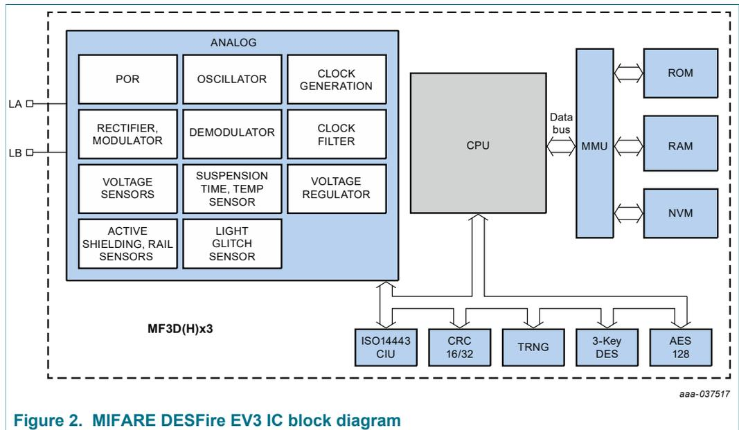
Figure 2. MIFARE DESFire EV3 IC block diagram
